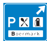
K3 Information sign for exit to motorway service area, showing the name of the rest area and symbols for the services offered
