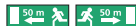
L19 Nearest exit or second nearest exits in the directions and at the distances indicated on the sign
